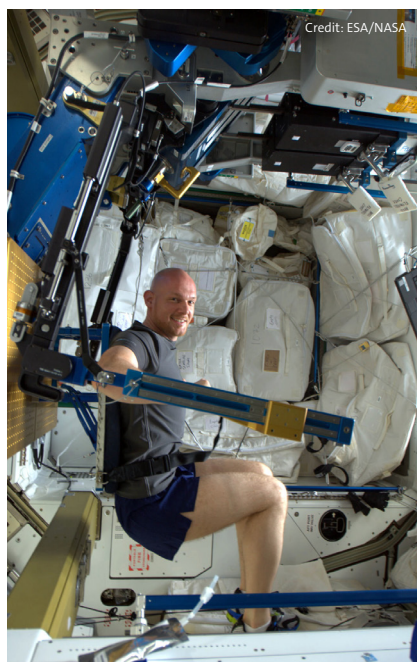
↑ ESA astronaut Alexander Gerst uses the International Space Station's Advanced Resistive Exercise Device (ARED) to stay fit by simulating weightlifting using air pressure instead of traditional weights.
